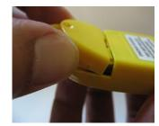
6. Replace cover, as shown. Cover will snap into place. Replace screw.
