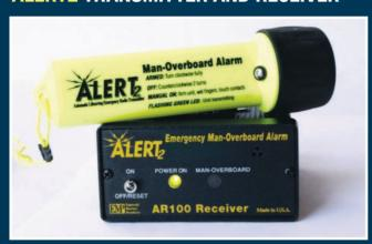
When a crew member falls overboard, the water-activated ALERT2 Transmitter sends a radio signal to the ALERT2 On-Board Receiver, sounding a 95 dB alarm and marking your position on a compatible GPS. The ALERT2 Receiver can be wired to shut-down an engine - offering an impressive margin of safety for the single-handed operator. Certified Intrinsically Safe model of the ALERT2 Transmitter for hazardous locations also available.
