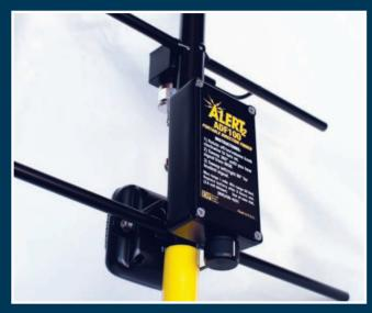
The ALERT2 Portable Direction Finder is a rugged hand-held navigational antenna, allowing the user to search for the ALERT2 Transmitter signal by manually sweeping the horizon while monitoring the spray tight loud speaker.
